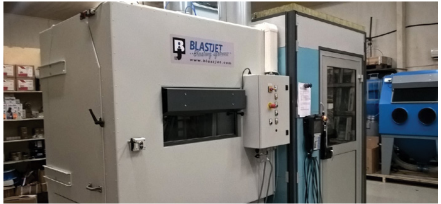
Finland-based Blastjet specializes in abrasive blasting systems. It has developed a robotic system for use in wheel and brake shops that removes paint from rims.
