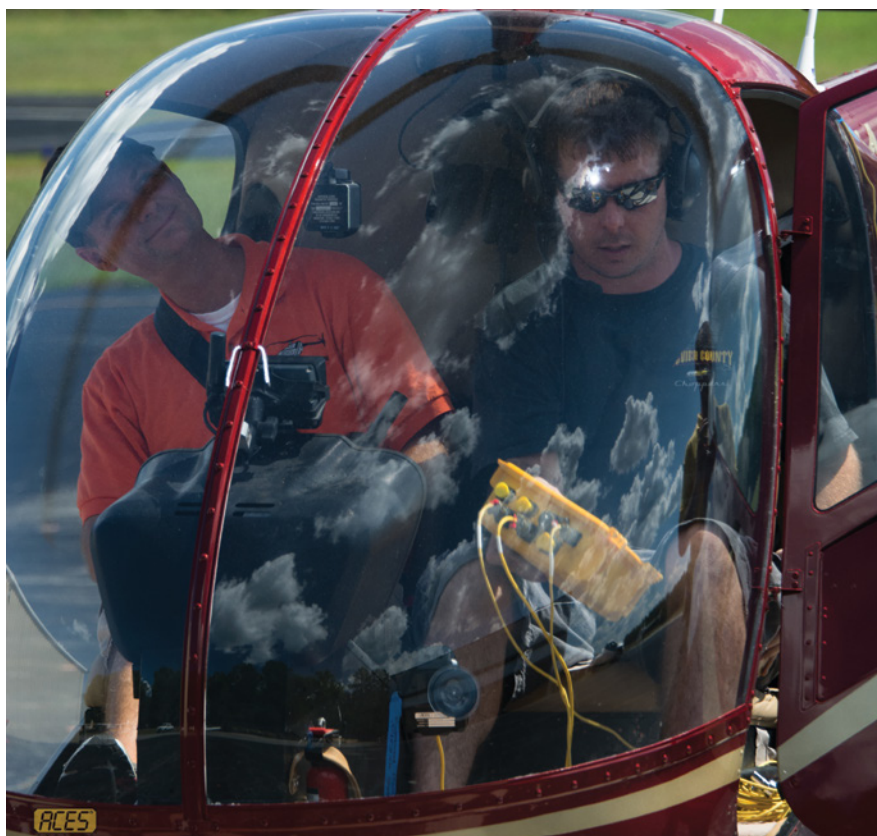
Operating the ACES analyzer in an R44. A learning algorithm in the ACES Systems allows the unit to become smarter with each successful track and balance run, according to Chris Mullins, EVP of Marketing and Product Support for the company. Aces image.
