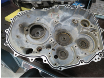
Corrosion damage or blocked filters can lead to expensive unscheduled maintenance of components such as the integrated drive generator. Shown here is the IDG housing. ExxonMobil image.
