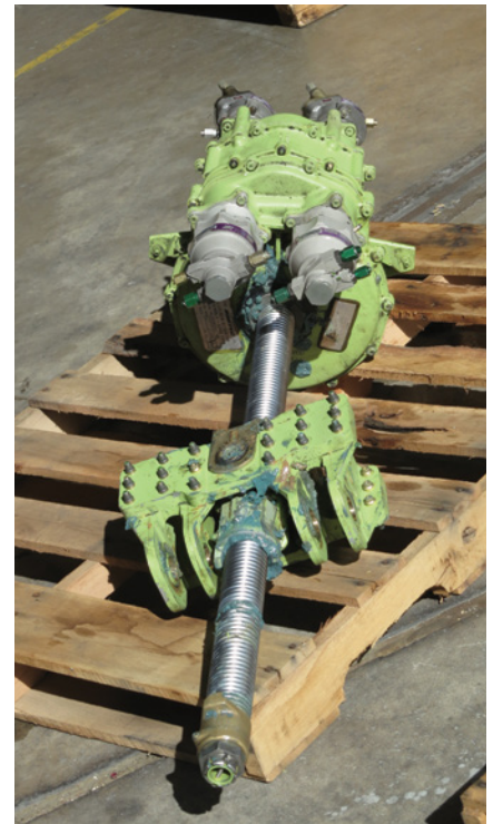
Insufficient lubrication of components like this jackscrew assembly can lead to excessive wear and ultimately thread failure. This was found to be the cause of the Alaska Airlines Flight 261 accident in 2000. ExxonMobil image.
