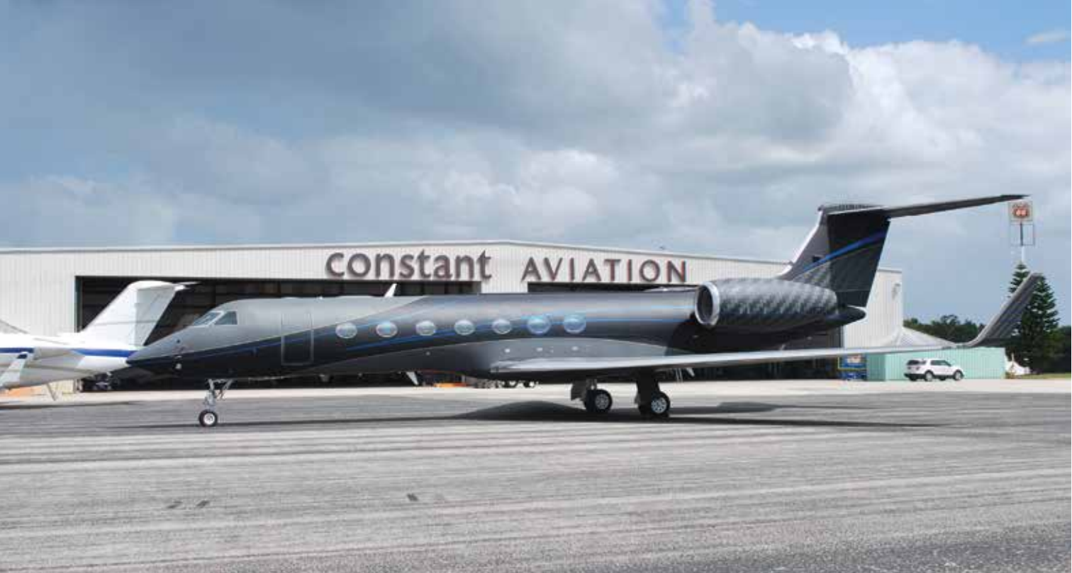
Specialty matte paint from Sherwin-Williams Aerospace Coatings made for a unique look on this Gulfstream. The only gloss paint is the pinstriping between the "carbon fiber effect" on the nacelles, tail and winglets and the blue accent striping. The scheme was laid out by hand. Constant Aviation image.
