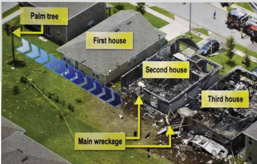
Aerial photograph showing the main wreckage and impacted homes. The blue arrows show the general westerly direction of the airplane's travel at impact. The aircraft struck the palm tree shown in the upper left-hand corner of this photograph. (NTSB Photo)
