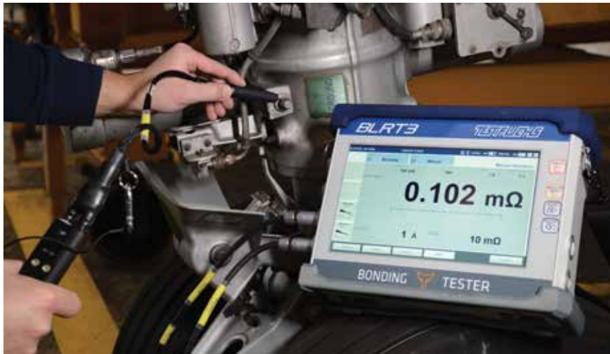
IFS and TEST-FUCHS are exploring new areas for implementing digital twins by using test equipment to gather data like resistance and impedance on parts such as hydraulic valves. IFS/TEST-FUCHS image.
