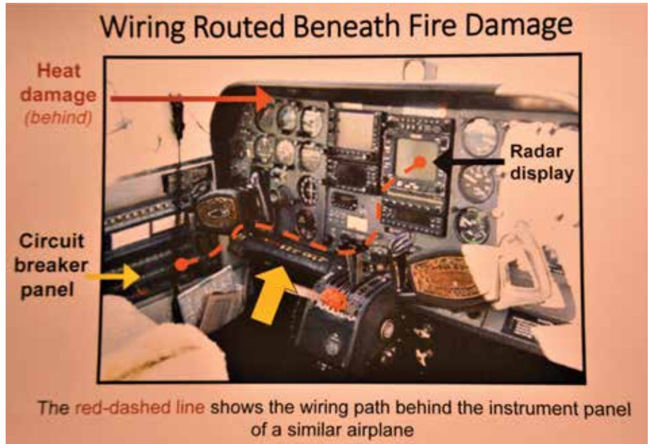
This photo shows the instrument panel of an exemplar Cessna 310R that had a similar configuration as the accident airplane. The location of the radar display and circuit breaker are shown. The dashed line portrays how the wiring was routed between the two. (NTSB Photo)
