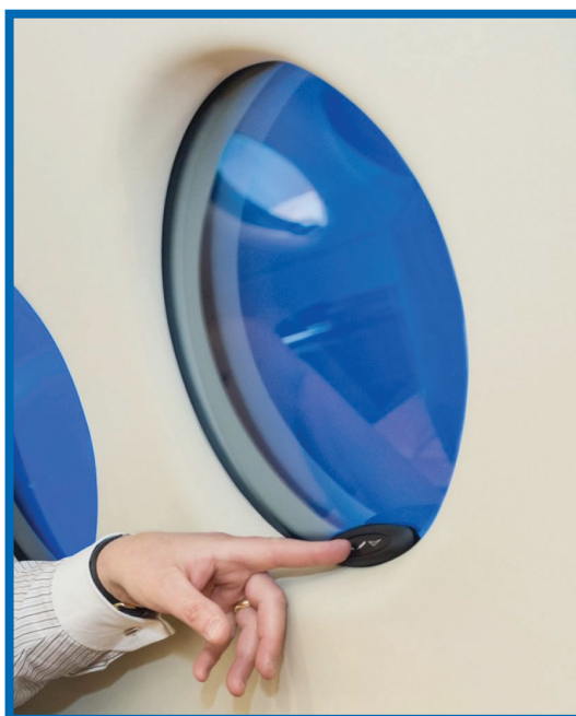
SPD-SmartGlass windows can be in tuned on a window-by-window basis so that each passenger can get the exact amount of light they are looking for. Research Frontiers image.
