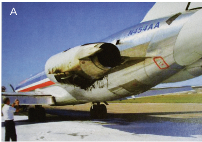
Investigator documents the left engine damage following the emergency landing.
