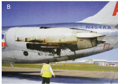
Side view of fire-damaged left engine damage.
