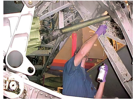
Zip-Chem recommends assessing the condition of every airframe and powerplant for corrosion issues prior to parking it. Zip-Chem image.
