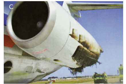
Close-up view (looking aft) of the left engine after the fire was extinguished by Airport Rescue and Fire Fighters (ARFF).
