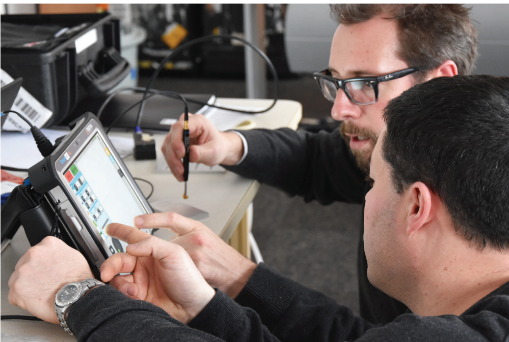
Testia calls their Smart UE1 product “the Swiss-army knife of NDT inspectors.” They say this wireless, light-weight device (2kg) offers both ultrasonic and eddy current testing capabilities in a single device. Testia image.
