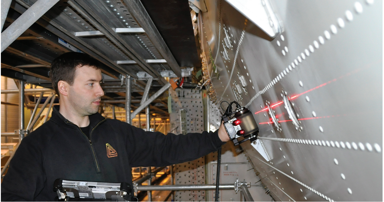
Testia says its Thickness Tool helps make efficiency leaps in the hangar. It has a phased array ultrasonic testing (PAUT) roller probe and includes acquisition, analysis and reporting software for super quick thickness measurements after blending areas of corrosion. Testia image.
