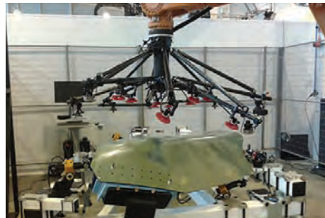
Automated manufacture of a STeM winglet box structure.
