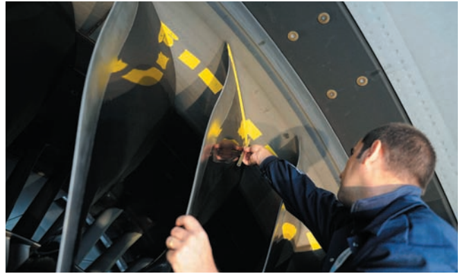
Claude Dubois, an AFI KLM E&M technician, created an innovative process that enables on-wing erosion measurements of the abrasion shroud found on GE90-110B/115B engines. AFI KLM E&M photo by Patrick Delapierre.
