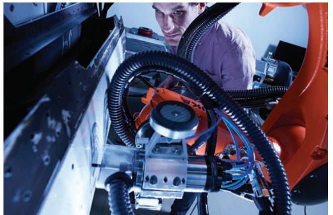
A multi-year research project at Lufthansa Technik resulted in a rapid repair process for composite structures. Once the repair process was determined, further development adapted that process, enabling mobile application of the new repair method. The end result is significant cost reductions. Lufthansa Technik photo.
