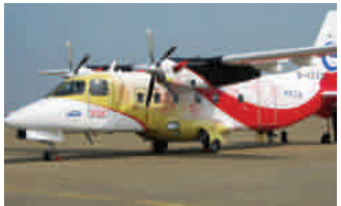
The Y12F, manufactured by Hafei Aviation Industry Co., Ltd., in Harbin City, Heilongjiang Province, features Hartzell props.
