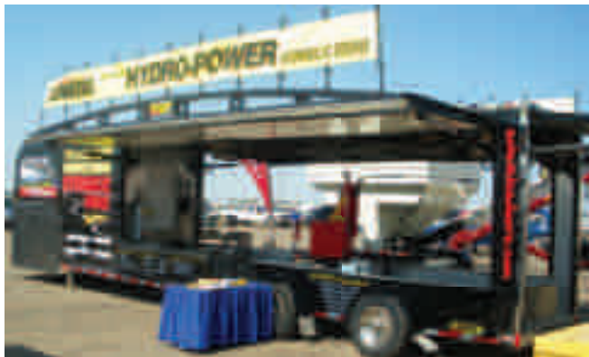
A large container has endless possibilities after attaching hydraulic doors to the side or endwalls. Schweiss Doors show trailer has hydraulic doors that open up the sides. It allows set up and take down in a matter of minutes.
