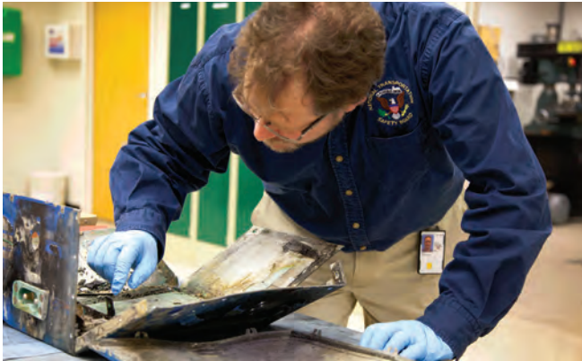
NTSB Materials Engineer Matt Fox examines the casing from the battery involved in the JAL Boeing 787 fire incident
