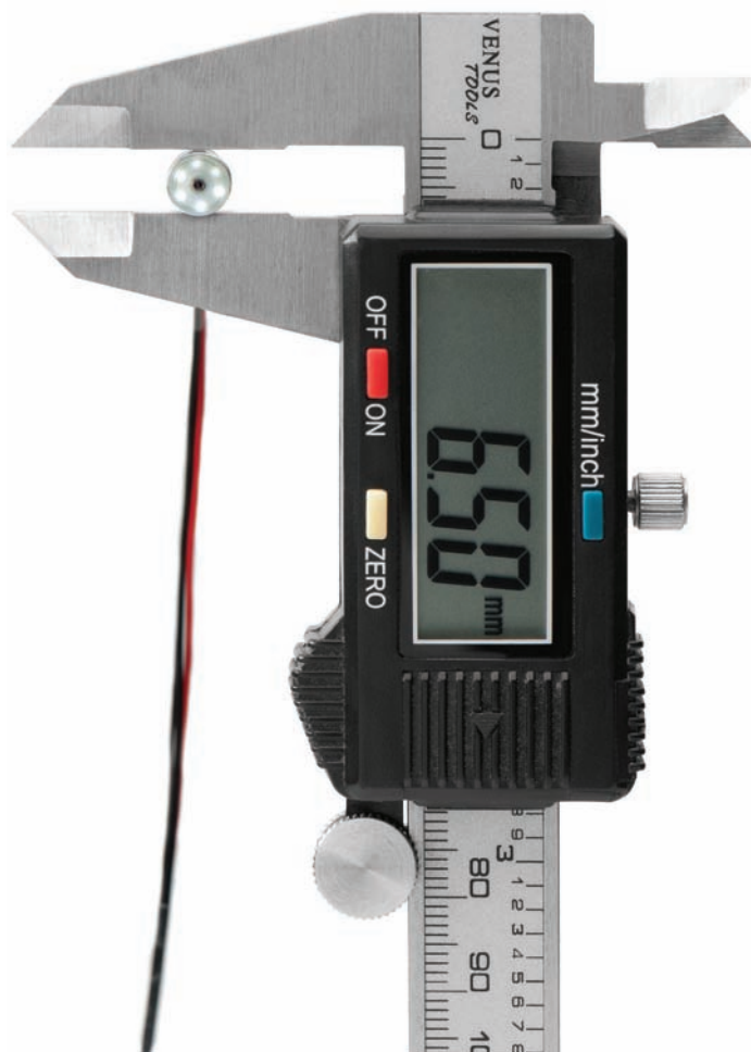
The micro ScoutCam 6.5 Lum camera was initially developed for a robotic refueling mission in outer space. Medigus Photo.
