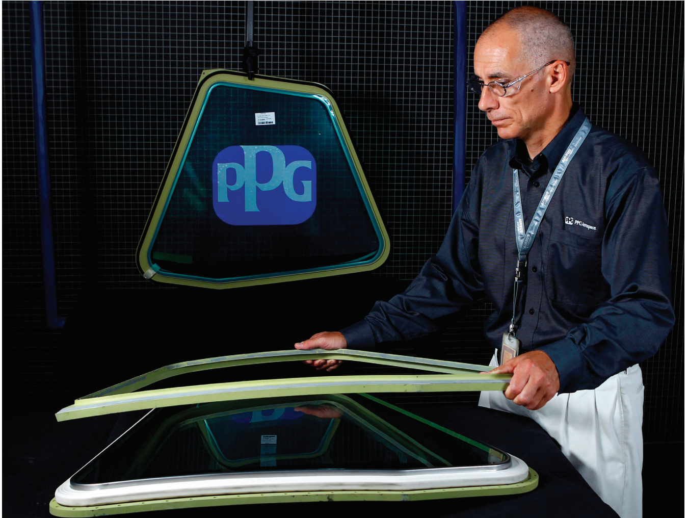
Frame Retainer is removed from a sliding cockpit window for the Airbus A320 Family by Jim Hartmann, PPG Industries program manager, that PPG has redesigned. The new design enables the frame retainer and window panel to be installed as a complete assembly while being distinct components, affording cost-effective replacement. PPG offers framed window assemblies as well as window panels and frame retainer kits. PPG image.
