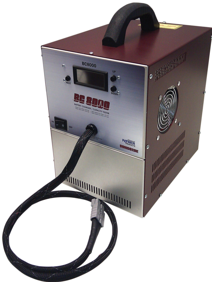
This COFKO BC-8000 unit can capacity-test, discharge-test and charge batteries. It comes with a power supply mode, used to charge aircraft emergency battery systems that have internal chargers. It monitors voltage, current, and time. Concorde Image.
