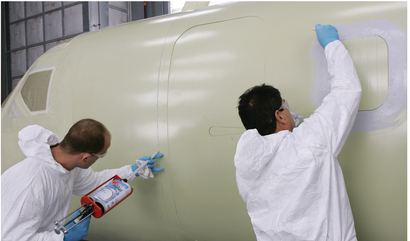
Basecoat/clearcoat technology potentially adds two to three years to the life of an aircraft's finish says Richard Giles, Global Technical Service and Training Manager, Sherwin-Williams Aerospace Coatings. Sherwin-Williams images.
