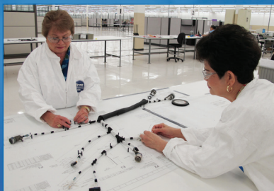
Wiring Harness & Electrical Cable Manufacturing
