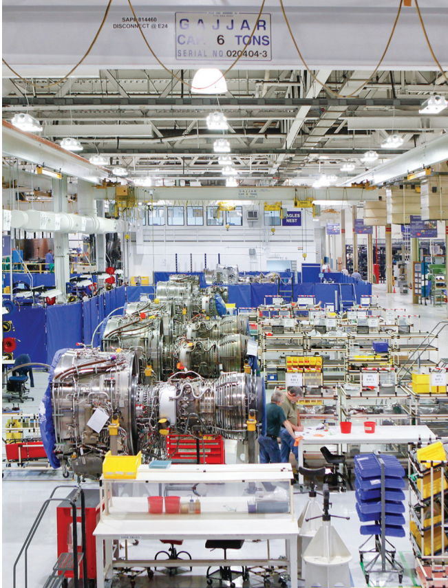
Mechanics overhaul V2500 engines at the Pratt & Whitney Columbus Engine Center in Columbus, GA.
