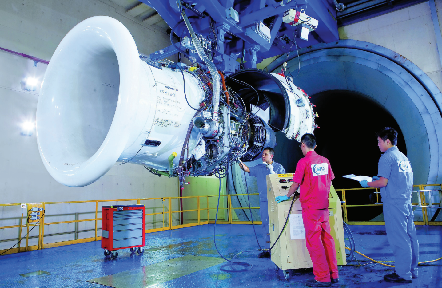
A CFM56-3 being prepared in the test cell at MTU maintenance Zhuhai, China, home to MTU Maintenance for the CFM56 family.
