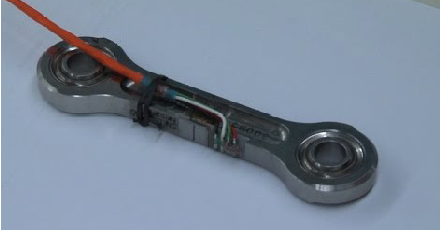
The MV-22B Osprey has tested a 3D-printed critical component in the engine nacelle. The 3D printed titanium link helps hold the engine onto the wing (there are four links per engine; only one was 3D printed during the test). (Photo: U.S. Navy)
