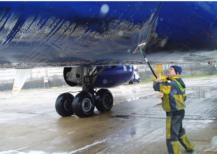
David Heissenbuttel, director of sales, Celeste Industries states that a dry wash system can be applied with a mop and removed to clean underneath an aircraft. (Photo: Celeste Industries)
