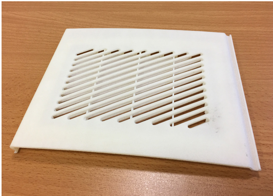
TEG's 3D-printed plastic speaker grill panel for a Jetstream 41 commuter aircraft which is certified with EASA Form 1. (Photo: TEG)
