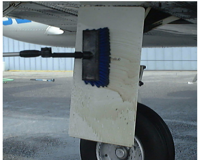
David Heissenbuttel, director of sales, Celeste Industries states that a dry wash system can be applied with a mop and removed to clean underneath an aircraft. (Photo: Celeste Industries)
