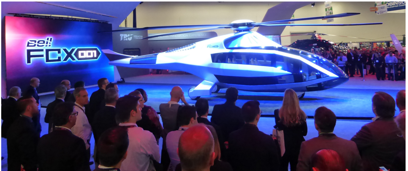
The main reveal at Heli-Expo was Bell Helicopter's FCX001 Future Concept helicopter. Features would include morphing main rotor blade tips, multiple fans in the tail-boom for anti-torque, and augmented reality cockpit. (Photo: ATP)
