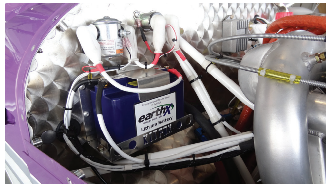
This aviation battery is installed in a Kitfox plane. EarthX Lithium Batteries image
