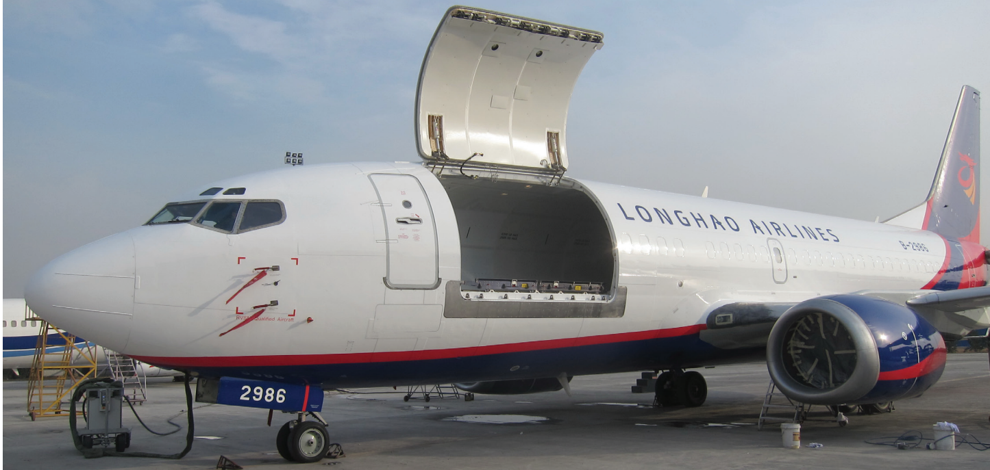
Pemco World Air Services (PEMCO) has redelivered its first B737-300 passenger-to-freighter converted aircraft to Guangdong Long Hao Aviation Group. It features nine pallet positions, up to 43,100 pounds of payload, 4,600 cubic feet of total volume, and a max range exceeding 2,000 miles. (Photo: PEMCO)
