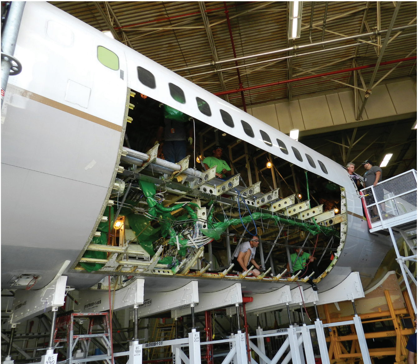
One of the first tasks in Precision's B757-200PCF main cargo door installation is the lower sill removal and replacement. Precision manufactures its own main cargo door. (Photo: Precision Aircraft Services)
