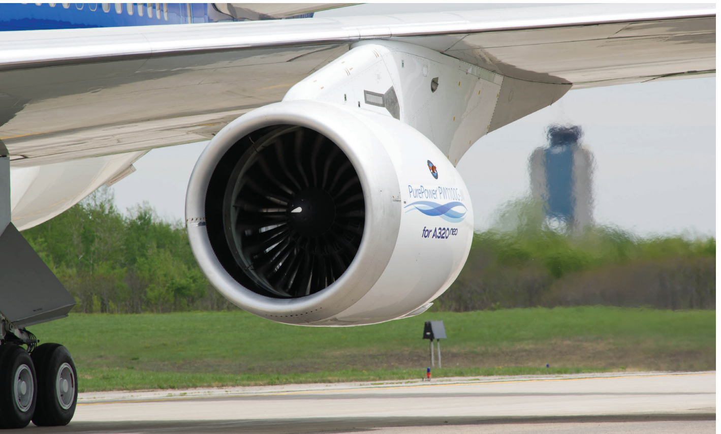
P&W's Geared Turbofan (GTF) family (such as the PW1100G-JM pictured) incorporates 40 percent more health and performance monitoring sensors than the V2500. (PW Image)
