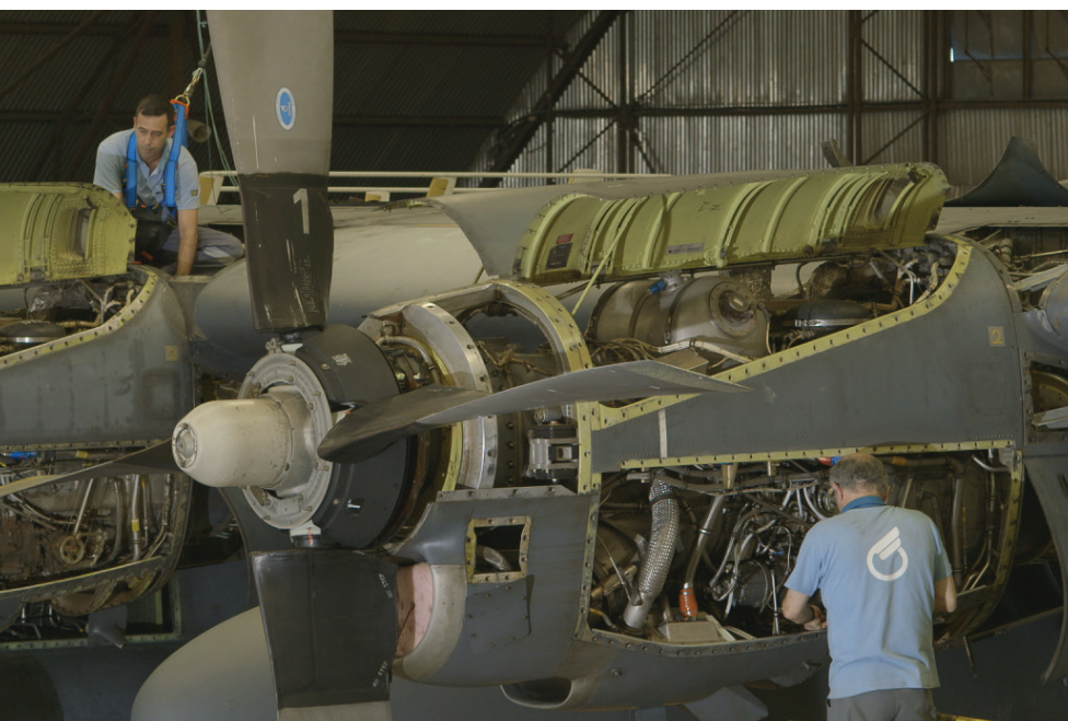
Top: An Embraer Legacy undergoing maintenance in the OGMA Executive Jets Centre. Above: OGMA engineers work on a C-130's T56 turboprop engines. (Photos: OGMA).
