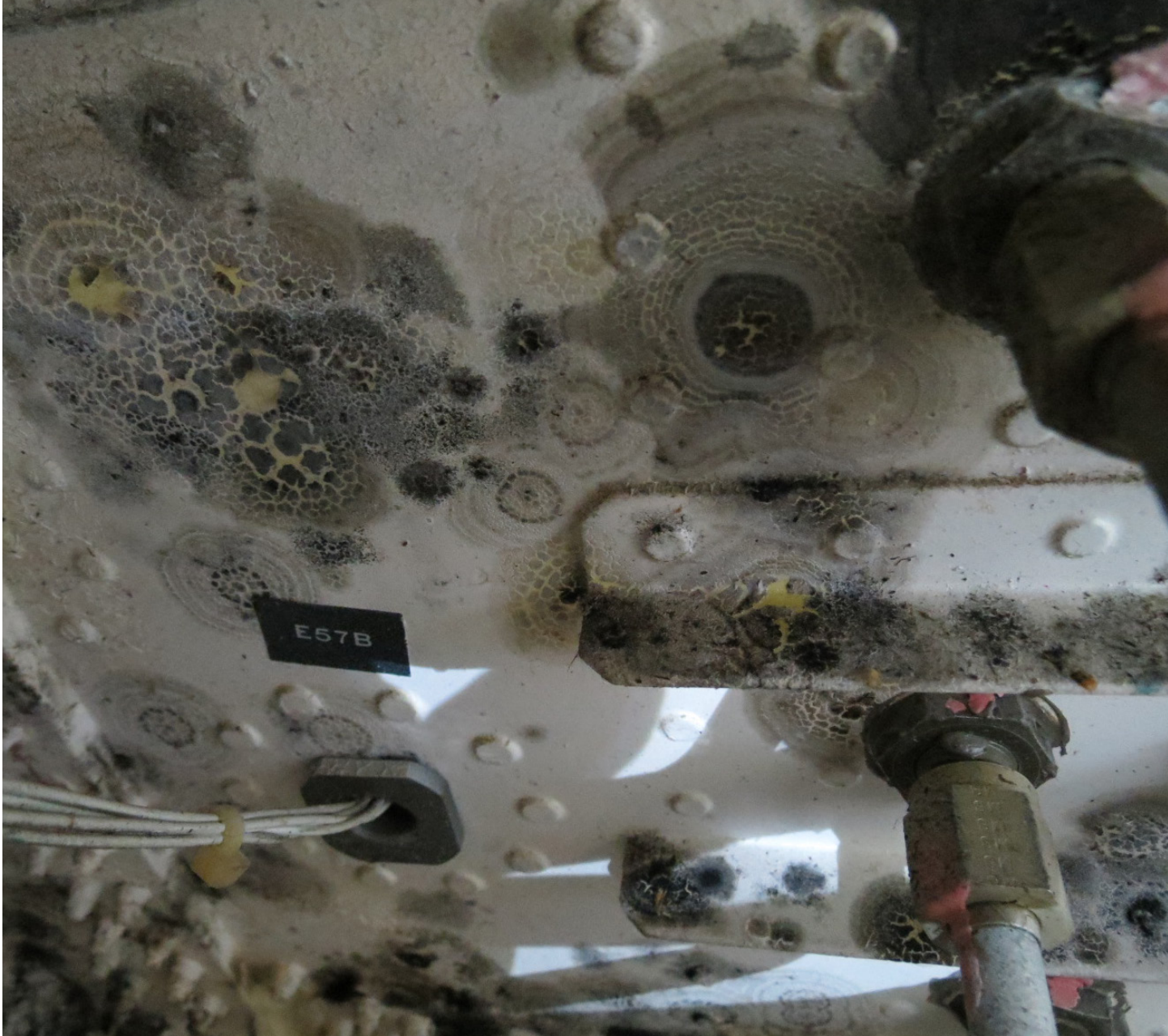
This close in shot shows how fungal contamination in an aircraft compartment degrades a polyurethane topcoat. U.S. Air Force photo/Dr. Wendy Goodson.
