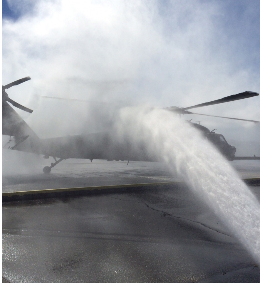
Riveer's Tactical Rinse System, an above ground, clear water rinse system in use with the U. S. Army at Hunter Army Airfield. (Riveer image.)
