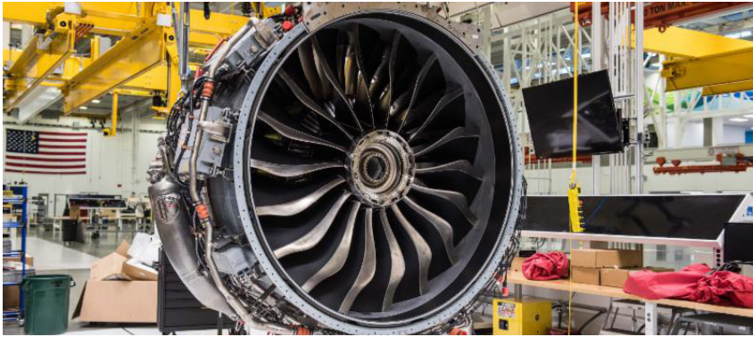
are engaged in full disassembly of LEAP engines as part of field inspection programs
