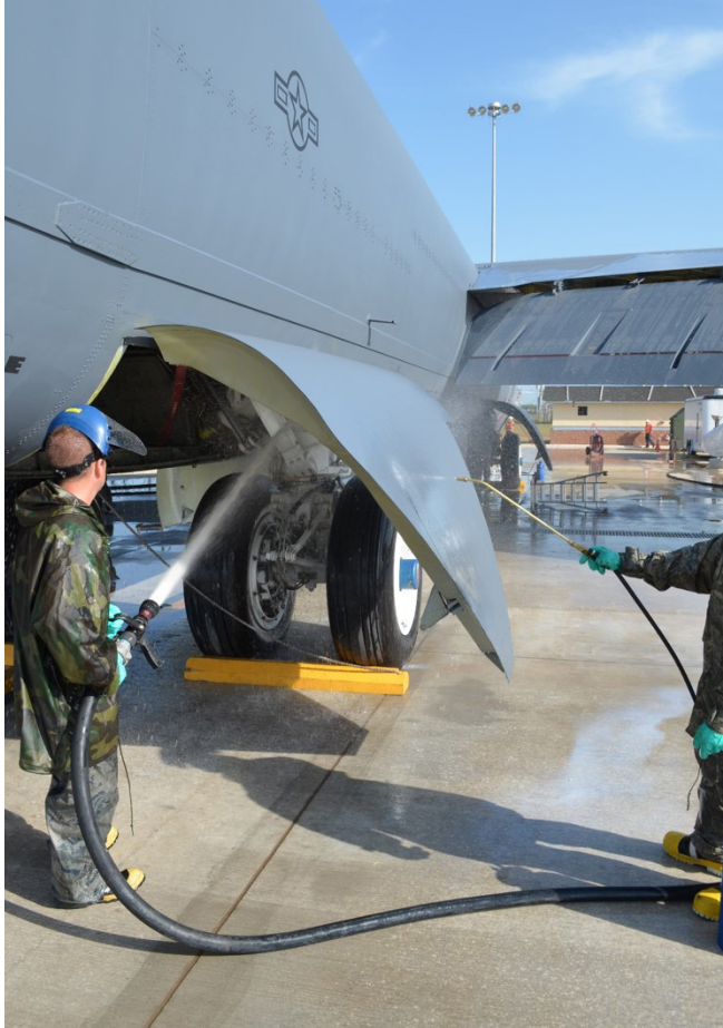
Riveer Environmental provides automated clear-water rinsing systems (CWRS). Shown is a B-52 wash system installed at Barksdale AFB in Louisiana. Riveer image.
