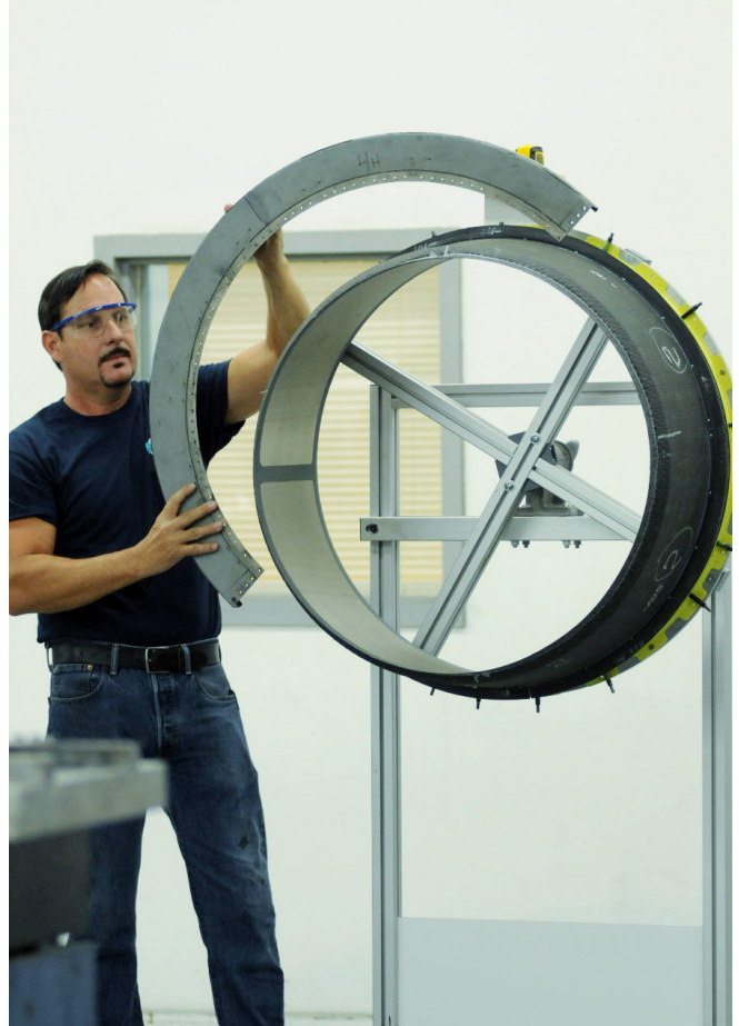
A composite inner barrel is added to the original inlet cowling's outer skin, lip skin and attachment flange on a Lear 60 aircraft. QTA image.
