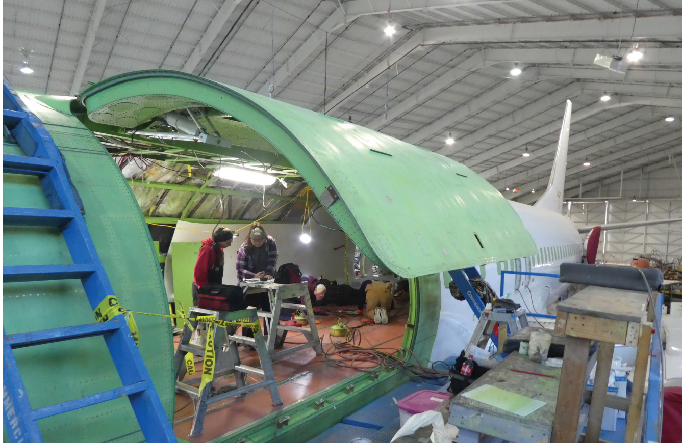
This cargo door by Aeronautical Engineers is hydraulically operated and actuated from the inside of the aircraft by an independent system. The door control and hydraulic panel are located on the 9g barrier, allowing a single person to operate the door. Aeronautical Engineers image.
