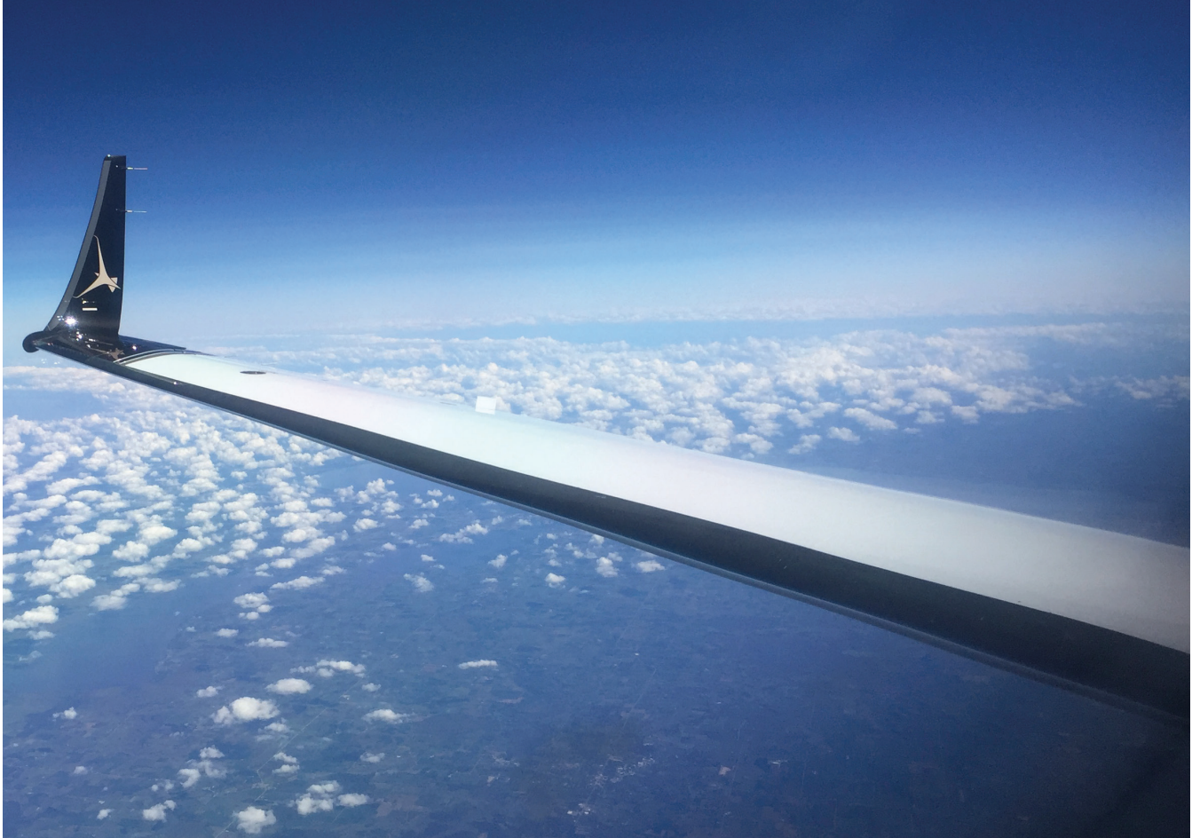
In cruise or normal flight, the winglets move little, if at all, only reacting to alleviate loads as they occur. Tamarack image.
