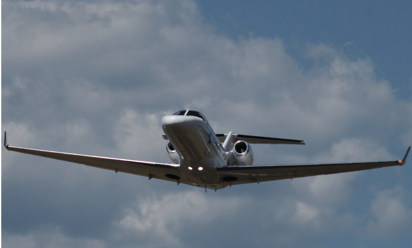
Within the active winglet, ATLAS, TACS or Tamarack Active Camber Surface, appears and functions like a small aileron, moving up and down. Instead of controlling flight maneuvers from pilot input, the TACS serves by reducing bending loads on the wing, and works automatically. Tamarack image.
