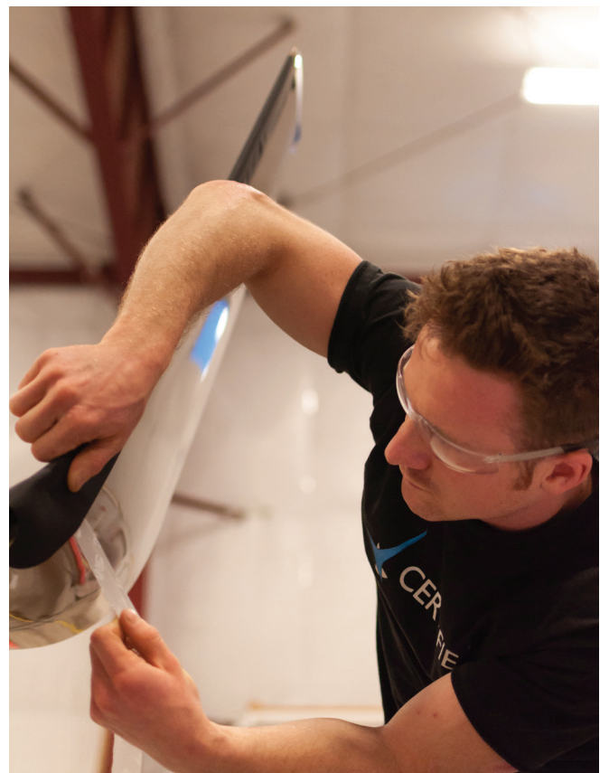
A technician works the attachment of a winglet. No specialized tools are required, except for a dedicated jig. Tamarack image.
