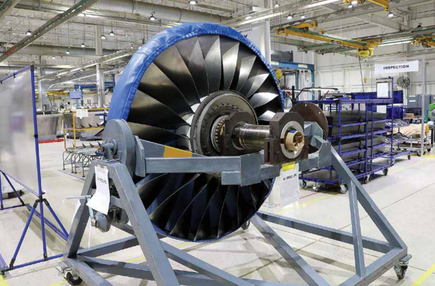
Material management is one critical factor in delivering responsive turn-around times (TATs) according to Max Allen, vice president of Commercial Programs RB211 for StandardAero. Shown above is an RB211-535 compressor. StandardAero image.
