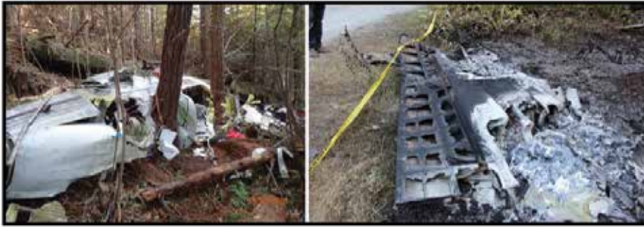
The left half of this photo shows the center fuselage wreckage from the inflight breakup of a Piper PA-31T airplane. No thermal damage was found. However, the forward fuselage and circuit breaker panels shown in the right half of the photo were severely burned due to a fire that was ignited by a chaffed electrical wire.
