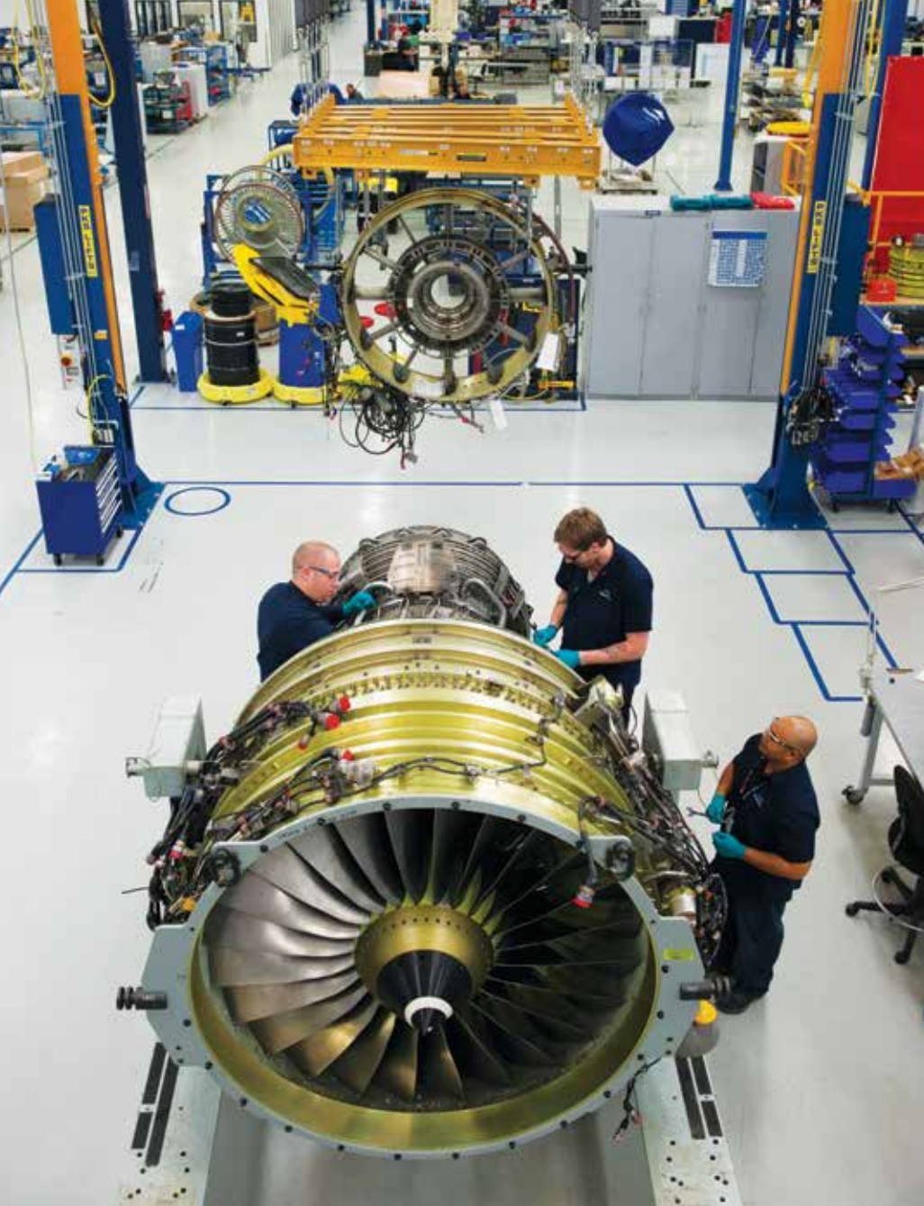
StandardAero says the North American market is rebounding strongly after the downturn of 2020, and this is driving a significant uptick in shop visits. Shown here is a CFM56-7B. StandardAero image.
