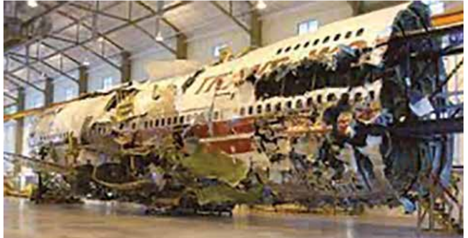
The 3-dimensional reconstruction of the wreckage from TWA flight 800 is currently housed at the NTSB Training Center. The reconstruction assisted investigators in determining that the center wing fuel tank exploded, likely due to deteriorated wiring in the fuel quantity indicating system (FQIS)
