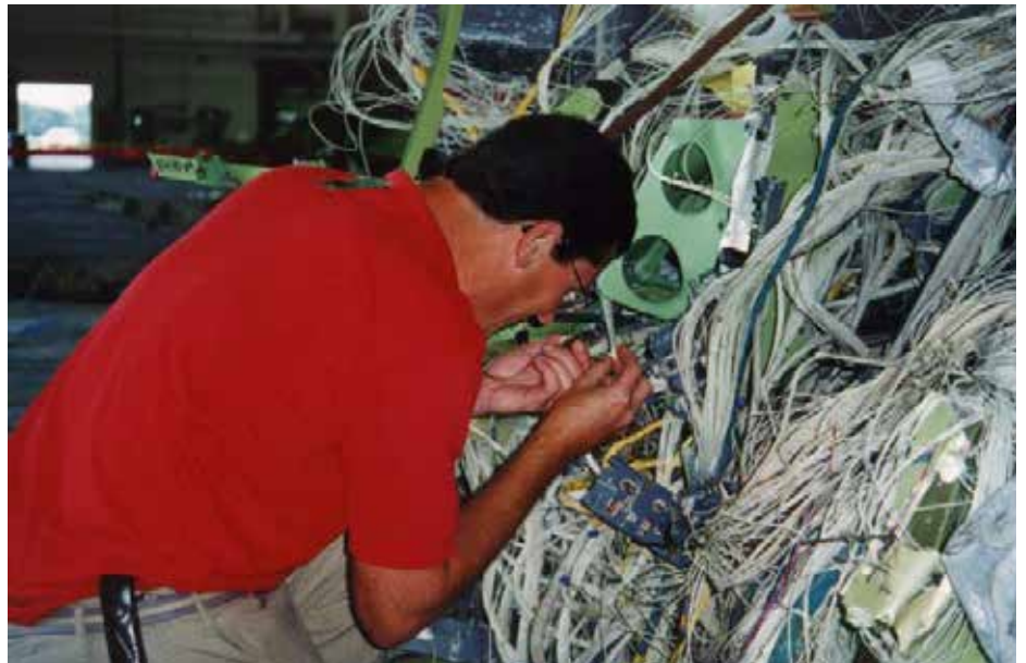
NTSB systems investigator Bob Swaim shown here examining the damaged wiring from the TWA 800 wreckage and other similar aircraft.
