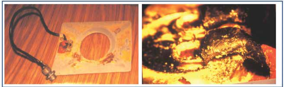
The static port heater plate from the MD-88 incident airplane. Note the magnified view on the right side of the graphic, showing a sharp bend radius of the lead wire around the thermostat case.
