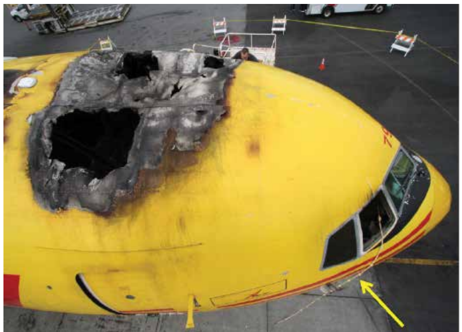
A view of the fire damage to the crown of an ABX 767-200 in San Francisco.
