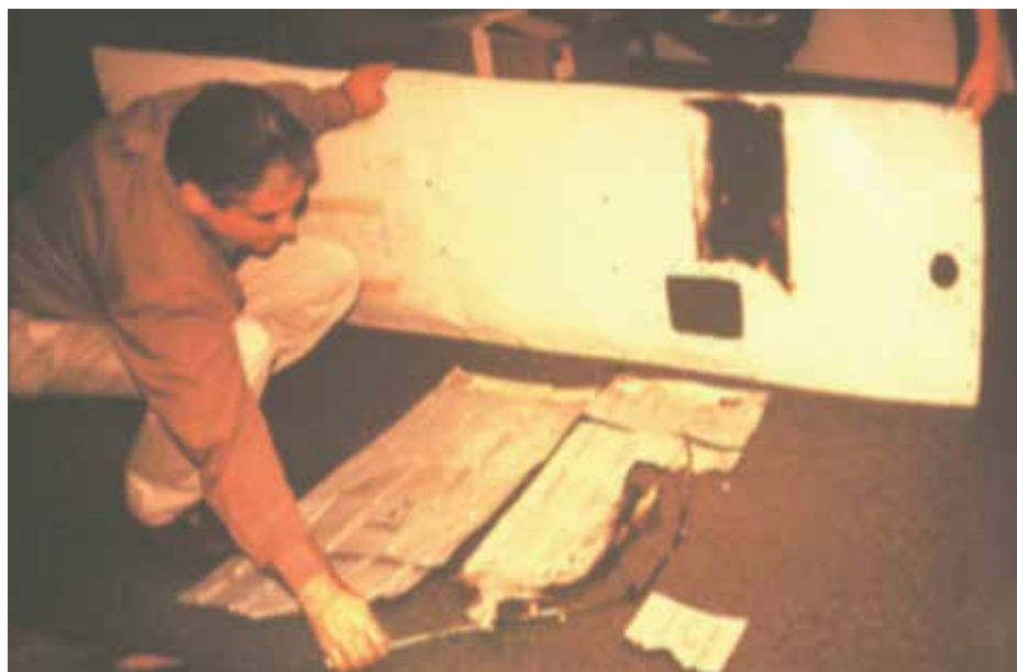
Investigators laid out the thermally damaged areas in the MD-88 cargo hold that were associated with the right-side static port.
