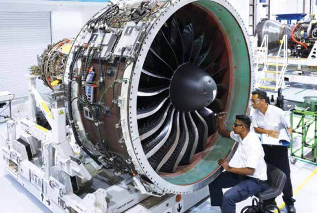
Pratt & Whitney's Eagle Service Asia facility in Singapore overhauls the fuel efficient GTF. Pratt & Whitney image.
