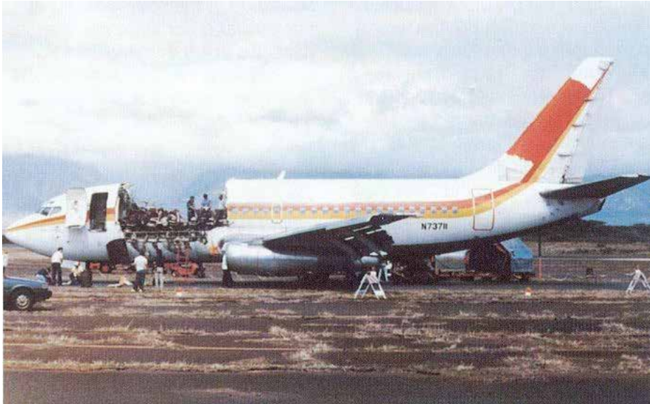
The NTSB said Aloha Airlines maintenance program failed to detect significant disbonding and fatigue damage that led to a lap joint failing. One flight attendant died and 65 of the 94 on board were injured. The image above shows the aircraft after landing on April 28, 1988. Image credit: https://ritkanlathatortotenelem.blog.hu/2013/12/16/aloaha_823 .
