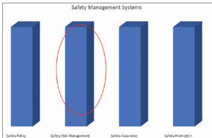
A safety risk management (SRM) system is one of the four key components of a complete Safety Management System (SMS).
