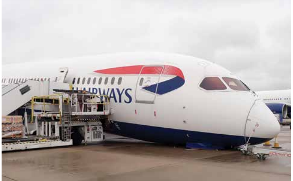
When the recovery operation lifted the nose of this British Airways 787, the downlock pin was found fitted not in its hole but in the apex pin bore next to it. This occurred after multiple checks to ensure the downlock pins were in place.
