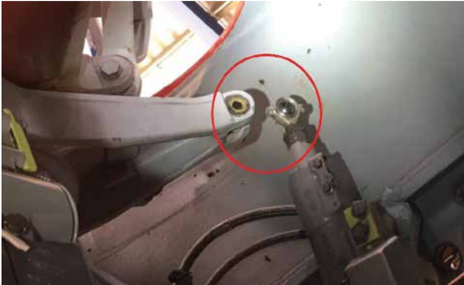
In this Northern HeliCopter AS365-N3 incident, the pilots found cyclic inputs had no effect on the rotor disk. After aborting the flight, they returned to the hangar and found that the left actuator was not connected to the swashplate that redirects the main rotor blades (see image above). Its fastener was missing. They found the bolt, two washers and one Nylon stop crown nut on the gear box compartment below. Operator, via BFU, images.
