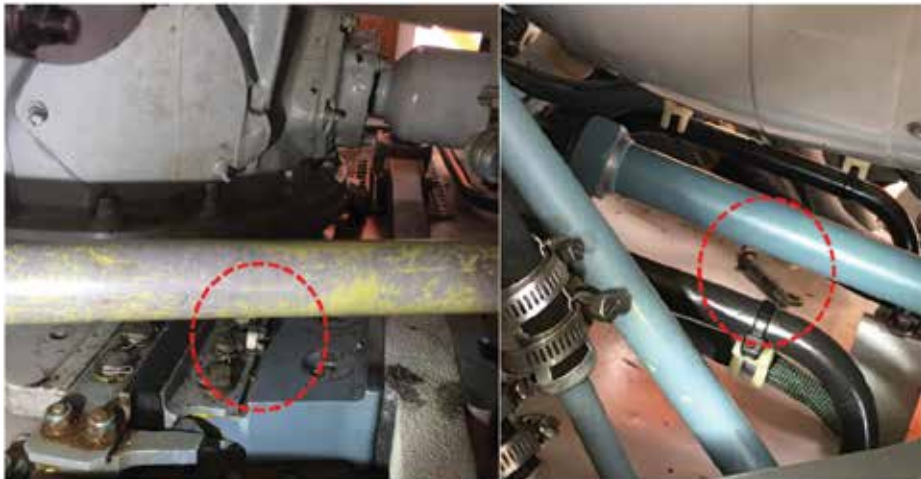
In this Northern HeliCopter AS365-N3 incident, the pilots found cyclic inputs had no effect on the rotor disk. After aborting the flight, they returned to the hangar and found that the left actuator was not connected to the swashplate that redirects the main rotor blades (see image above). Its fastener was missing. They found the bolt, two washers and one Nylon stop crown nut on the gear box compartment below. Operator, via BFU, images.
