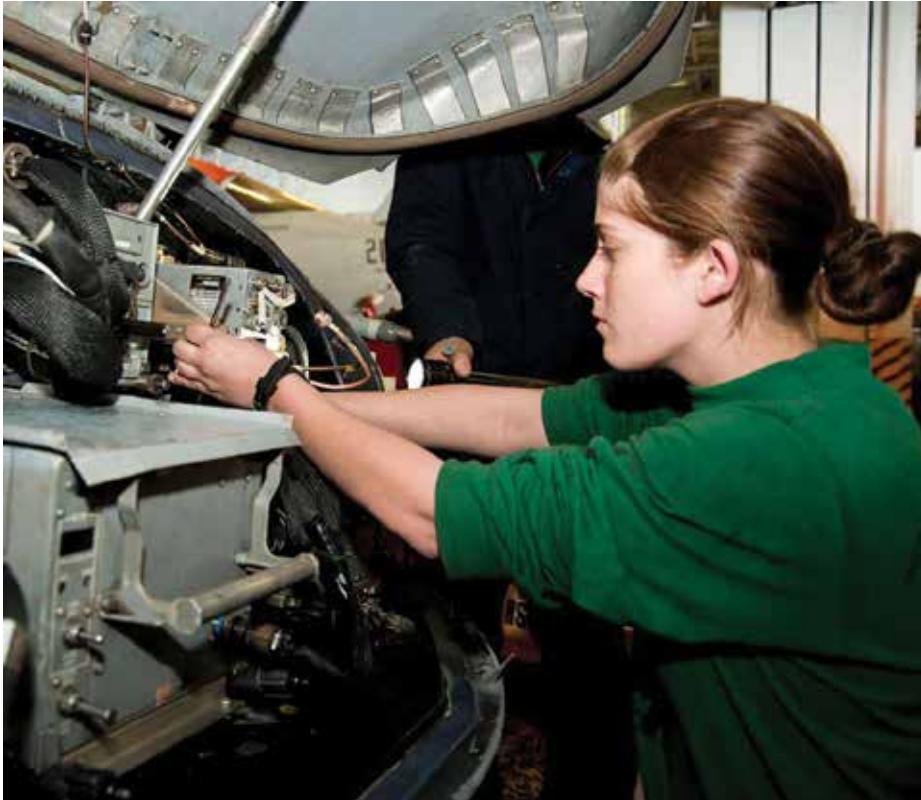
Aviation Structural Mechanic 2nd Class Jessica Neff replaces a radar altimeter on an SH-60F Sea Hawk helicopter. U. S. Navy photo by Mass Communication Specialist 3rd Class Britney Epps.
