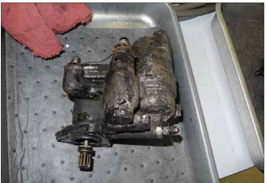
Graphic 8. The suspect fuel pump was removed from the engine by investigators and disassembled for clues.
