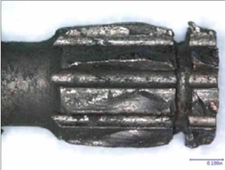
Graphic 9. Digital microscope photo of the damage to the internal splines of the drive gear after cleaning. The splines exhibited evidence of severe damage, with significant portions of the spline teeth missing material.
