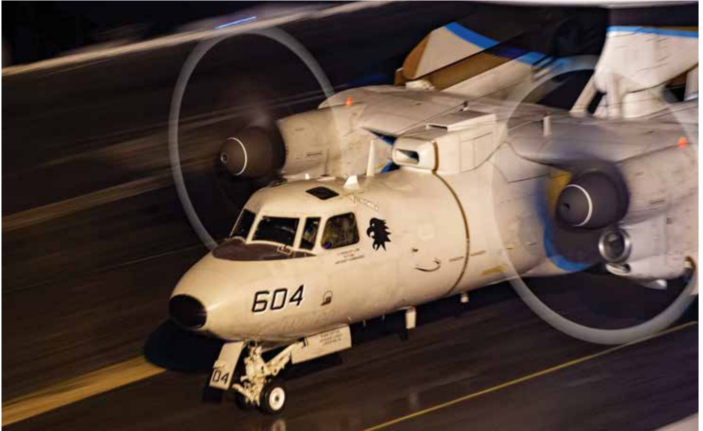
Sailors direct an E-2D Advanced Hawkeye assigned to the Black Eagles of Carrier Airborne Early Warning Squadron (VAW) 113 on the flight deck aboard Nimitz-class aircraft carrier USS Carl Vinson (CVN 70), Sept. 11, 2021 in the South China Sea. Seen on the propellers above is Sherwin-Williams AfterGlo photoluminescent paint. U.S. Navy photo by Mass Communication Specialist 3rd Class Jeff D. Kempton.
