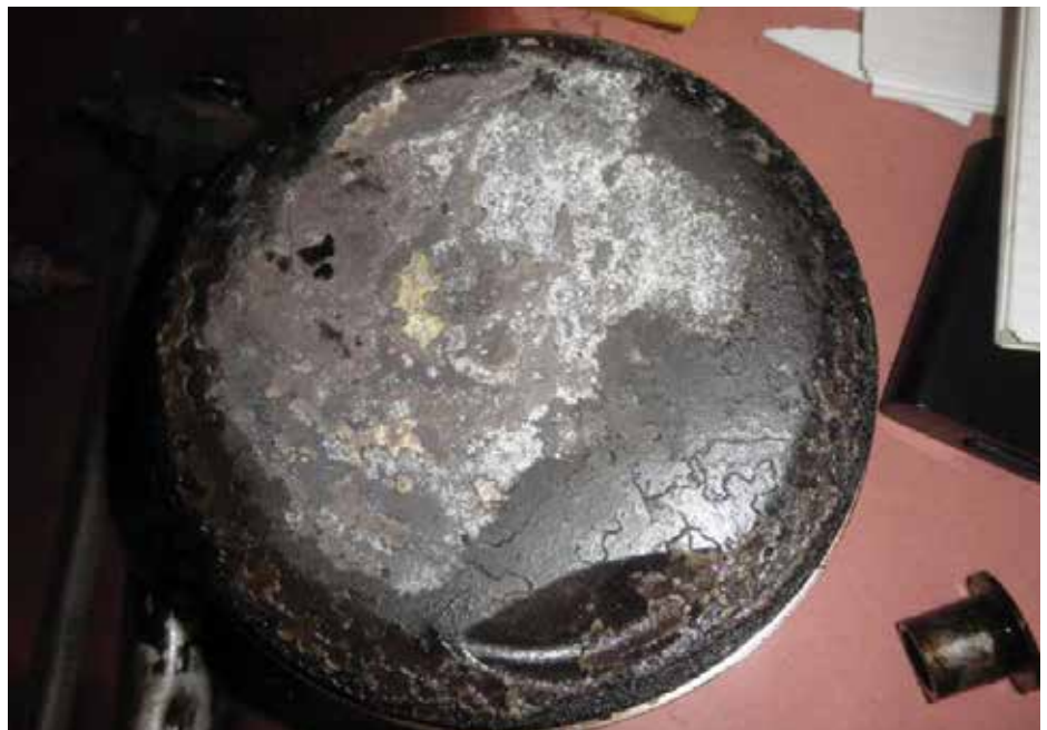
Photo 8: The no. 4 piston head of the No. 3 Engine, after it had been removed by investigators during the engine teardown. Note the whitish coloring and the damaged texture, indicative of detonation due to premature ignition.
