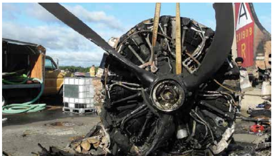
Photo 9: The No. 4 engine, as viewed at the accident site.
