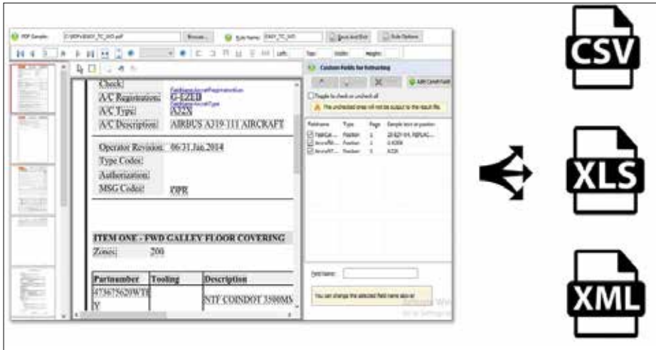
This image shows extraction for data from PDF through optical character recognition (OCR) technologies in Ramco's digital task cards. Ramco image.
