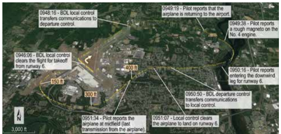
Photo 7: An aerial view of the traffic pattern flown by the Nine-O-Nine with the recorded ADS-B track and air traffic control communications overlaid.
