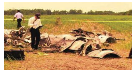
Graphic 2 – Final resting site of the main wreckage of the EMB-120. Pieces of the horizontal stabilizer were missing in this area.
