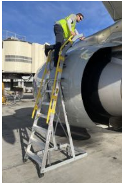
Cowl pylon ladders
