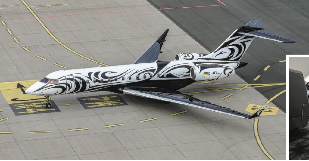
Project Pearl was a recent FAI cabin reconfiguration, avionics upgrade and a new and dramatic exterior paint scheme on a Global Express. FAI Technik images.
