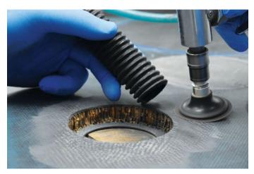
The taper scarf repair technique for composite structures is where a tapered cavity is machined into the damaged area, replacing the damaged material and providing a large, gradual surface area for bonding a new patch. This technique creates a joint with uniform shear properties, restoring the damaged composite structure to its designed strength and avoiding the need for external, bolted patches. Abaris image.
