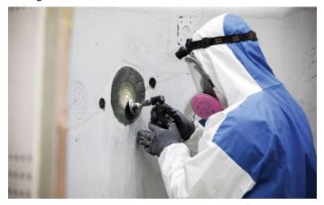
Advanced NDT methods produce more accurate mapping of the damage, new scarfing tools ensure repeatable and accurate repair geometries and portable hot bonding systems have improved, according to Vallair's François Fermaut. Abaris image.
