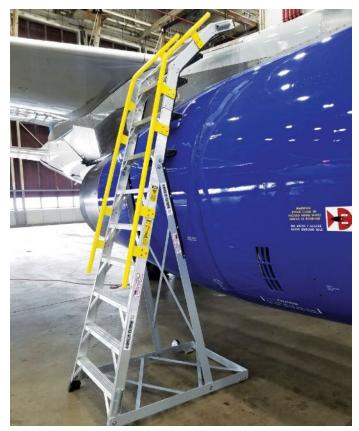
LockNClimb's 10 and 12 foot cowl pylon ladders allow technicians to quickly access maintenance panels on the top of the wing pylon area of Airbus and Boeing aircraft. LockNClimb image.
