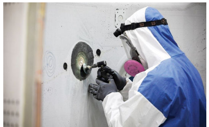
Advanced NDT methods produce more accurate mapping of the damage, new scarfing tools ensure repeatable and accurate repair geometries and portable hot bonding systems have improved, according to Vallair's François Fermaut. Abaris image.
