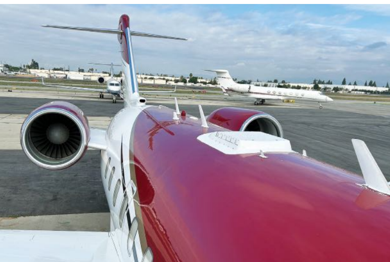
StandardAero generated the first pair of Gogo Galileo STCs for the HDX and FDX terminals on Challenger 600 series. This fuselage supports the Gogo Galileo FDX antenna.
