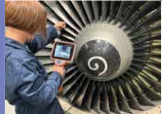
An inspection engineer performs an inspection using Waygate Technologies' Mentor Visual iQ+ borescope. Waygate Technologies and GE Aerospace have jointly developed a new AI-enhanced version that will be made available to customers through an upcoming software update for the Mentor Visual iQ+ video borescope later this year. GE Aerospace image.
