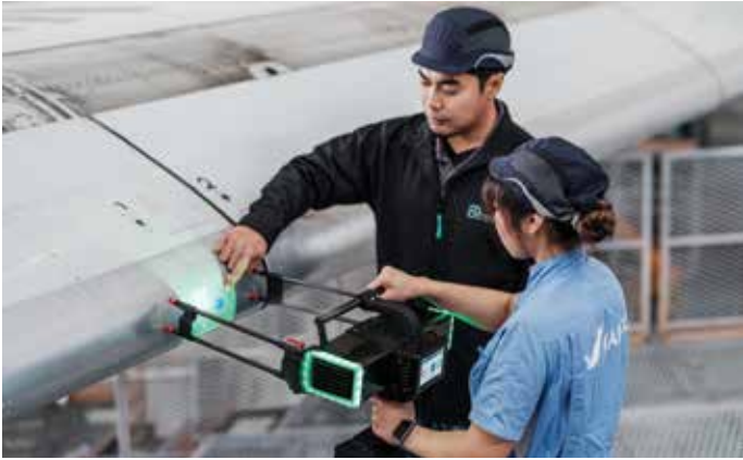
Smart inspection tools such as digital dent-mapping systems allow technicians to quickly measure damage on complex surfaces like wing leading edges, delivering accurate results through intuitive, easy-to-use workflows. 8tree image.
