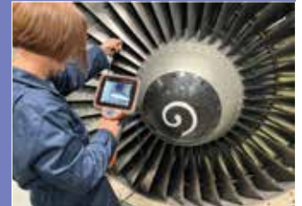
An inspection engineer performs an inspection using Waygate Technologies' Mentor Visual iQ+ borescope. Waygate Technologies and GE Aerospace have jointly developed a new AI-enhanced version that will be made available to customers through an upcoming software update for the Mentor Visual iQ+ video borescope later this year. GE Aerospace image.
